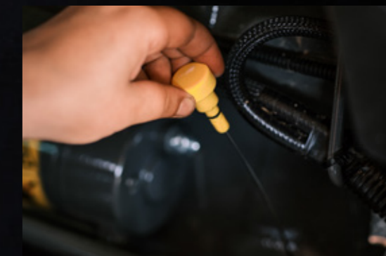
Front axle and slim waist bonnet design make oil dipstick and filter access easy.
